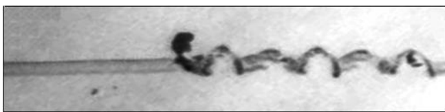
Fig. 4. Transition of a periodic track (period 45 microns) to a smooth one (or vice versa). Polycarbonate. Optical microscope [15]
