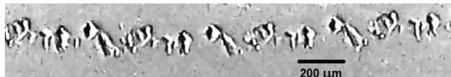
Fig. 16. Track on an X-ray film from a grain of quartz sand (optical microscope).
