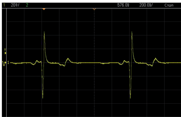
Fig. 13. The output signal of the reader circuit.
