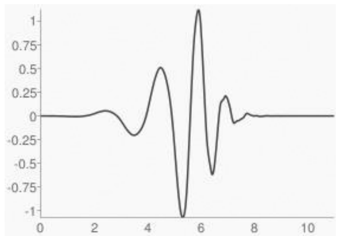
Fig. 3. The shape of the DB6 wavelet filter.
