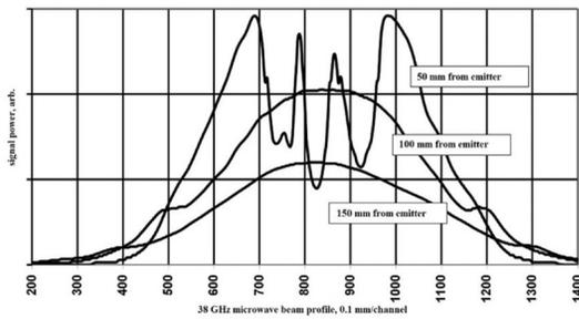
**Fig. 2.** Comparison of the shape of the 38 GHz microwave beam profiles (without taking into account the relative magnitude of the signal), depending on the distance from the transmitter to the receiver 50, 100 and 150 mm. Output horn diameter 45 mm, horn length 60 mm and input horn 35 mm, horn length 50 mm.
