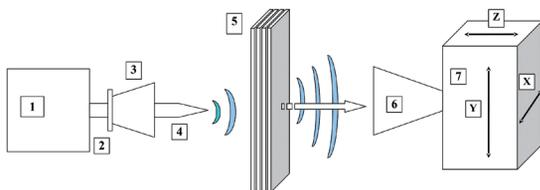
**Fig. 1.** Installation diagram. 1 - microwave radiation generator 38 GHz, 2-output horn antenna, 4 - Teflon dielectric insert of constant or variable cross section, 5 - dielectric sheet absorber of microwave radiation of variable thickness 0-50 mm, 6 - receiving horn with a microwave radiation receiver connected to the ADC and control computer, 7 - system of 3-dimensional X-Y-Z positioning of the receiver.
