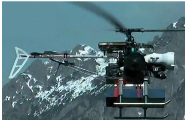
Fig. 1. Placement of the radiometer on the UAV.
