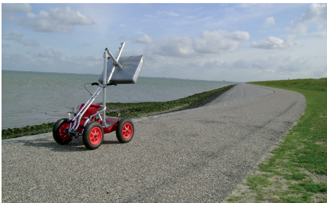
Fig. 4. Moving the radiometer on the trolley.
