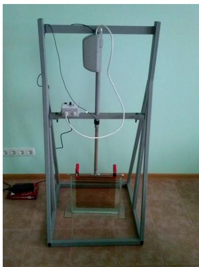
**Fig. 1.** Dip-coating device.
