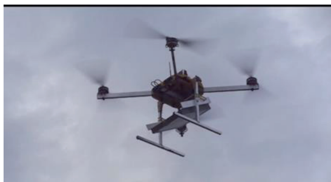
Fig. 1. The microwave radiometer on a quadcopter installation.
