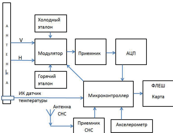
Fig. 3. The microwave radiometer with sensors block diagram.
