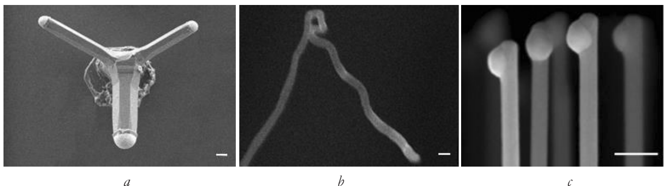
Fig. 3. Uncontrolled PEA growth: (a) NWC Si_xGe_{1-x} with droplet rupture and crystal branching, (b) Si NWs with bends, (c) InAs NWs with droplet migration to the side walls [11]. Scale bars 100 nm.
