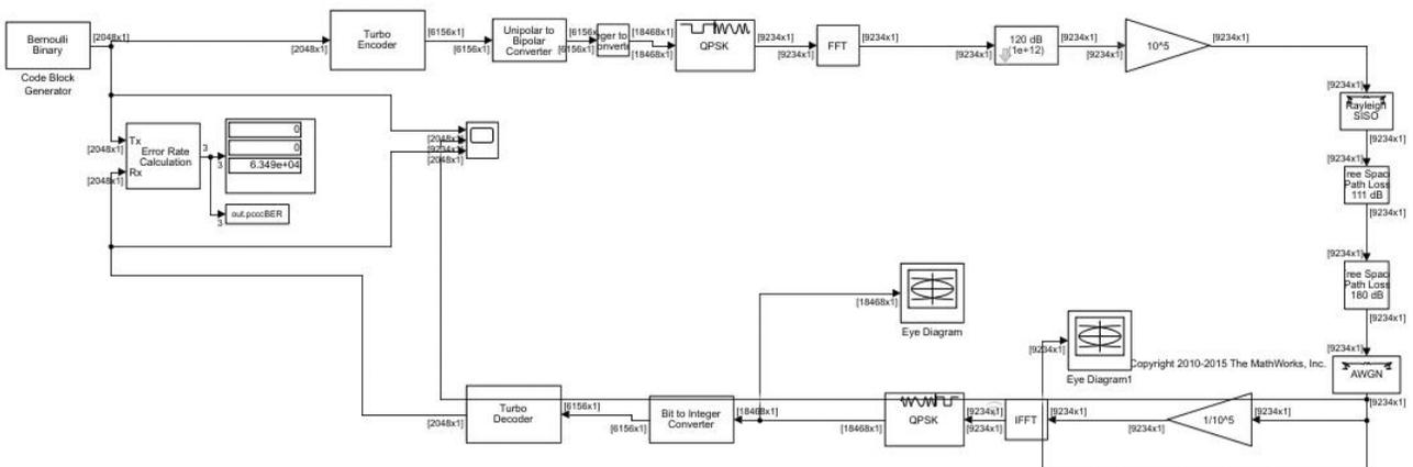
Fig. 1. Transceiver for data based on LTE standard.
