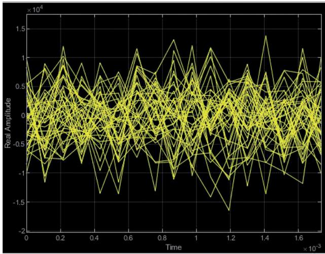
**Fig. 3.** The eye diagram of received signal SNR = -21 after AWGN channel.
